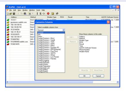
Using a template from Wireless ACE, you can change the configuration in several modems at the same time and can check and update their firmware as well. AceNet also features logging to a database and charting for the monitored modems.
